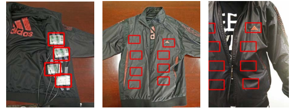
(a) Inside view (b) Front view (c) Worn on body Fig. 4: Wearable cloud jacket using Raspberry Pis.
